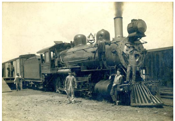
SAL RY class L-4, 4-6-0 #785, a 1907 product of Baldwin with inclined valve chests, has made a stop in Lake City on March 3, 1915 with west bound local #50. This locomotive was retired in 1923, but some of its sisters lasted into the late 1940s. - Donated by L. A. Bailey
