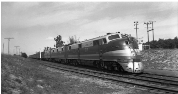
SAL's winter-season all-Pullman south bound Orange Blossom Special with nearly new A-B-A EMD E units and 15 heavy weights was making its stop in Sebring, FL in this 1941 scene. The water column was still in place for steam locomotives. The OBS was suspended for the duration of WWII after the 1941-42 season due to the need for Pullmans for troop trains. Sam Appleby photo, CFRHS collection .
