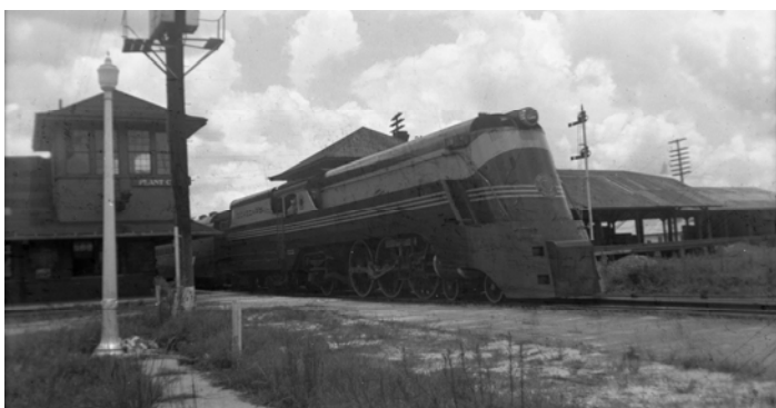
SAL's streamlined Pacific 868 crosses the diamond at Plant City in 1940 as it begins its westward curve towards Tampa Union Station with the west coast section of the Silver Meteor . Due to a diesel shortage caused by expanded Meteor service, the SAL streamlined several of their Pacific's to make this run from Wildwood to Tampa and St. Petersburg, but they didn't carry the Silver Meteor nameplate. Sam Appleby photo, CFRHS collection .
