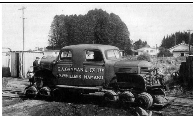
Home-Made Logging Road Engine. Photo Courtesy of ACL-SAL HS.
